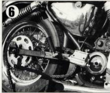
6 Install the new pulley onto the shaft with the flange facing out. Install the new nut and tighten it to 65-75 ft-lb. The new pulley uses the same set screw system as the old sprocket to keep the nut from loosening.
