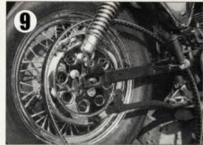
9 Place the belt over the rear pulley and, with your buddy helping, lift the wheel into place. Coat the axle with anti-seize and push it through from the left side of the swingarm. Install the washer and nut, hand tight only. Then drape the belt over the tranny pulley.
