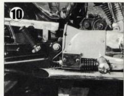
10 You can now install the kit's debris guard. This mounts under the swingarm with the supplied hardware. The new upper chrome belt guard mounts in place of the old chain guard. Then reinstall the front foot peg, brake pedal, and master cylinder. The bike can then be removed from the blocks and set on level pavement.
