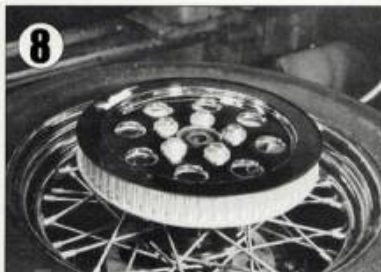
8 Bolt the new pulley to the wheel using the five supplied 7/16" x 14 x 1/2" bolts. The flange on the new pulley should face the wheel with the chrome cover on the outside as shown.
