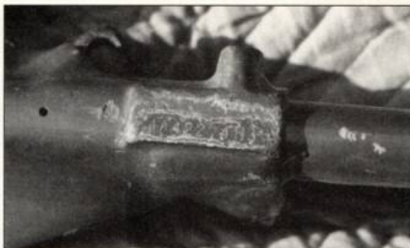
3 Here is the frame's VIN on the frame boss located on the right side of the neck, just above the downtube. These characters have the same style and coding system as the engine VIN.
