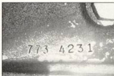
4 Another way to tell if the cases have been tagged is to check the crankcase numbers.
