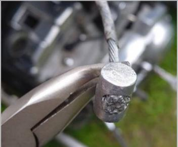
Note: The smaller hole in the barrel must be slightly bigger than the cable diameter. This will allow the tips of the bent strands to be caught in the hole. Pull on the barrel with all the tips inserted, then it must be tapped all the way in until it sits flush with the barrel. Solder will just secure the strands in place.
