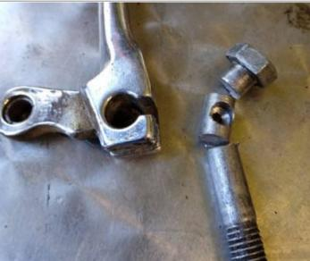
Today I've lost patience searching for fancy stuff (epoxies, etc.). Each wire of the cable end is turned back 180° and pulled back into the barrel. It locked itself in place. I have mounted like this into the lever on the bar. It worked great, not moving at all. Then I soldered. This way, I'm not dependig on the bond of the materials to give me confidence that it will last.
