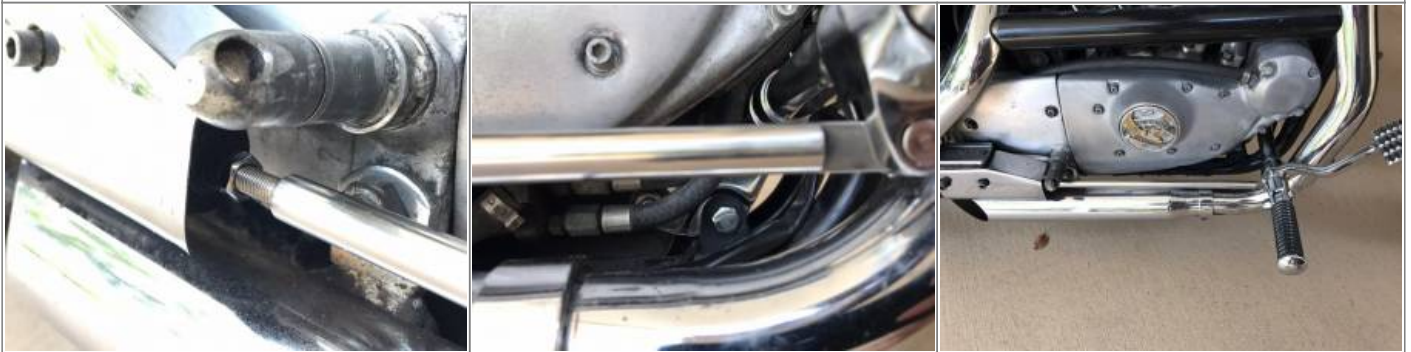
Hooking up the brake pedal. 7)
