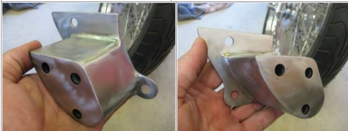
Custom made mounts to adapt BT forwards to a 77 model. 2)
