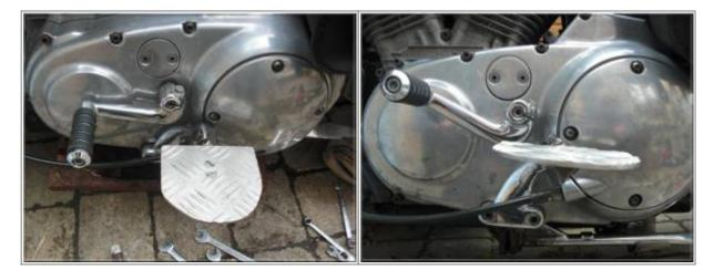
A short piece of square stock (scrap re-purposed here) with one corner flattened at a 45° for the peg mounts.
