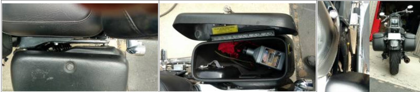
Leatherlyke Cruiser hard bags on a 2002 1250C. Dims: 7.5" Wide x 11.5" Tall x 18" Long. Hardware is quick release for easy bag removal. Keyed locking lid, closed cell neoprene liners, weather proofing seals, and necessary mounting hardware included. 3) 4)
