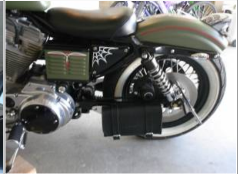
Bag mounted with chrome buttonheads, spacers and Loc-tite. 18)
