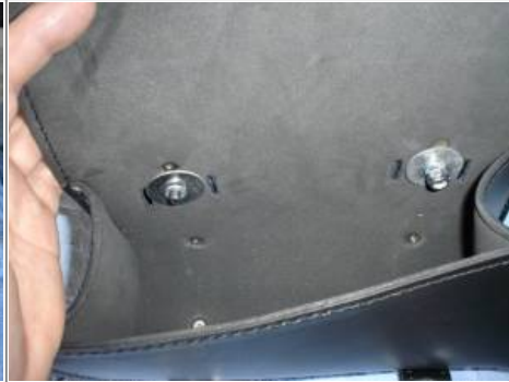
Inside the bag, large flat washers, lock washers and nylocks. 17)
