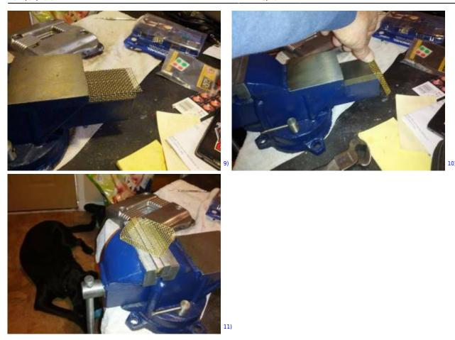
The inside bends ends had to be beveled back some to make room to shove it down the hole. Once it's bent properly, it can be installed with a little RTV silicon on the sides to help keep it in place.
