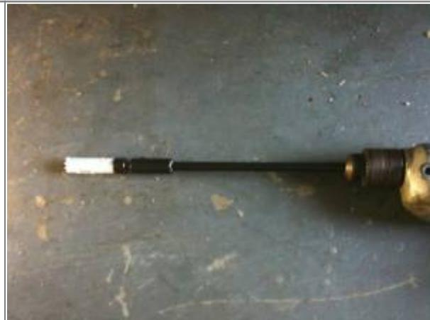
Drill out the center of the baffle (3/4" hole saw used here). <sup>10)</sup>
