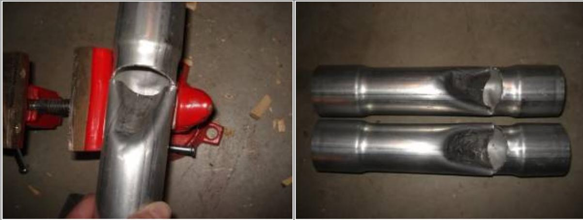
Drill holes in the baffle to let the diverted exhaust get back out.
