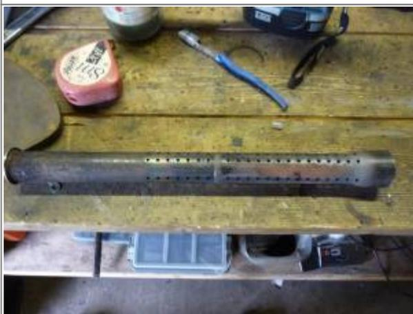
Holes in the baffle partially drilled out. <sup>24)</sup>
