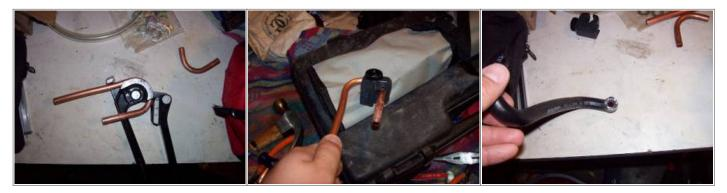
• After inserting the bends in the hose, cut the ends to length and install as usual.
