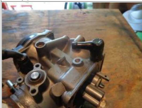
Keihin butterfly (non CV). Here is on way to do it. Break the plastic off and run a hose on the factory brass nipple. 27)
