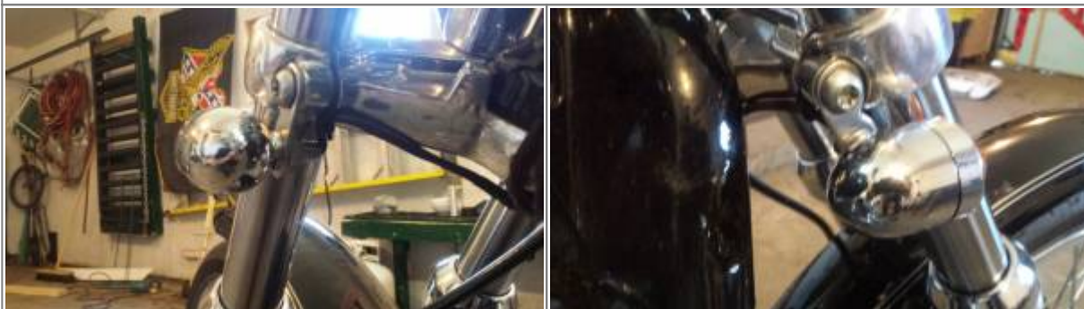
Bracket made from aluminum flat bar 24)
