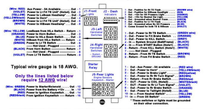
Note(1): The KILL Switch may be a momentary, normally-closed, switch or it may be a two position switch providing ON-OFF functions (like a rocker or toggle switch). It gets power from the the TH unit from J4-Pin3 (GREY wire). It MUST provide power to the TH unit on J4-Pin5 (WHITE) when not pressed and prevent power there when it is pressed. (Also see Note(2)) That WHITE wire must also be connected to one side of the START Button.
