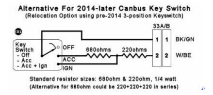
Be sure to carefully solder your connections and cover with shrinkwrap.
