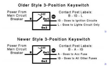
If you buy an older style switch (with B - IG - L functions) realize that you can use that switch on the later models, but the labels will not be correct for how you must connect it.
