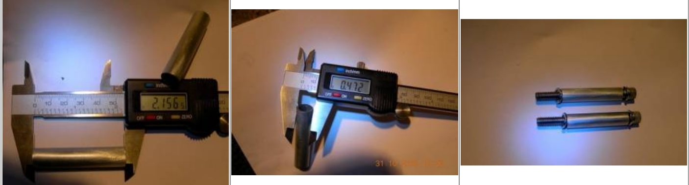
1/2" O.D.x1/4" I.D. sleeves slid over the bolts with washers under the head. Sleeves go between the eyebrow and the gauge housing. 15)
