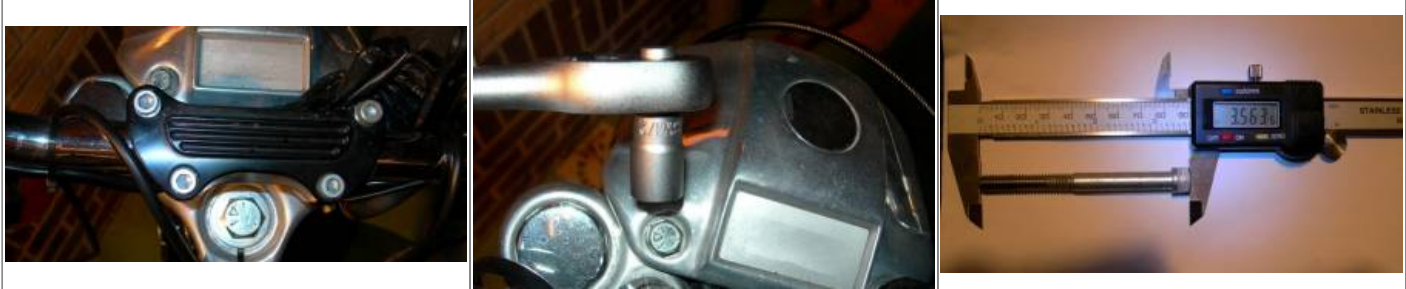
1/2" O.D.x1/4" I.D. sleeves slid over the bolts with washers under the head. Sleeves go between the eyebrow and the gauge housing. 15)
