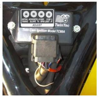
The TC88A has dials on the module for selecting pre-programed ignition timing maps and choosing the level of the RPM Limiter. This is accomplished with two dials for timing maps and two dials for the RPM Limit.
