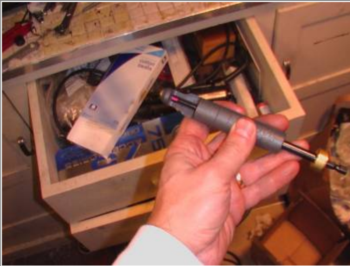
Install the helicoil with the insertion tool 7)
