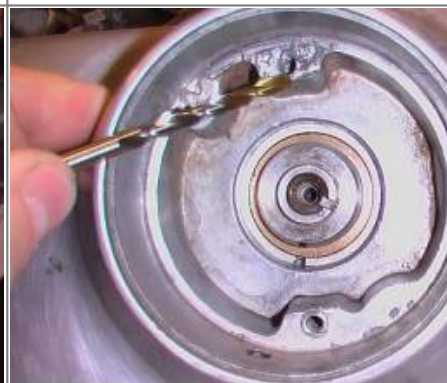
The proper drill bit is included to enlarge the hole (to make room for the Helicoil) 4)
