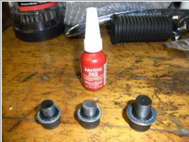
Zinc-plated O-ring washers with allen head bolts. Length cut to size. 40) 41)
