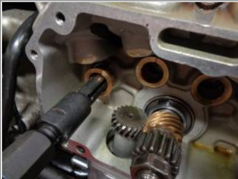
Hold outward pressure on the handle. Then yank the bushings out by knocking the slide against the handle end of the tool 5)
