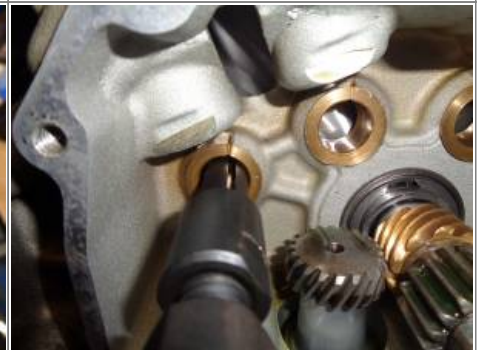
Hold outward pressure on the handle. Then yank the bushings out by knocking the slide against the handle end of the tool 5)
