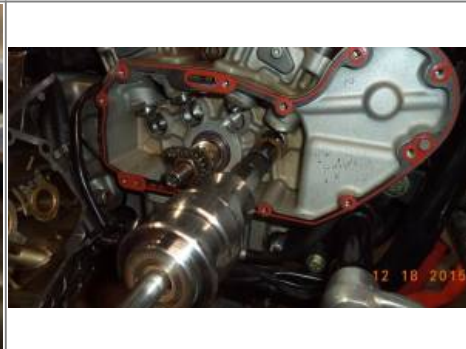
Hold outward pressure on the handle. Then yank the bushings out by knocking the slide against the handle end of the tool 5)
