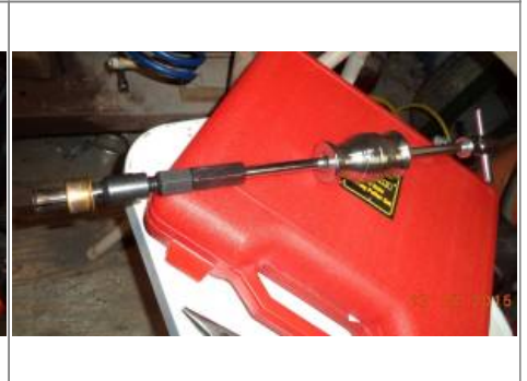
Hold outward pressure on the handle. Then yank the bushings out by knocking the slide against the handle end of the tool 5)
