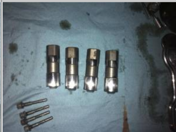
Notice how the wear ring extends down below the machined area of this S&S lifter a little. 20)
