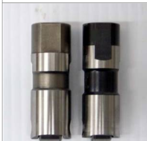
Note the much longer anti-rotation pin flats on a JIMS Lifter (right) This is required for high lift cams
