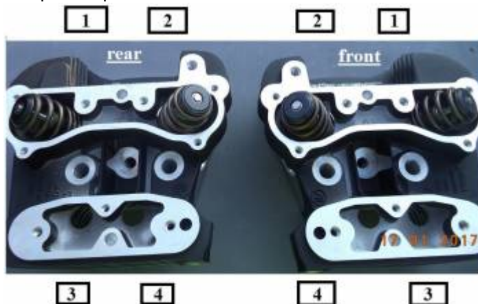
Head Bolt Removal and Installation Torque Sequence
