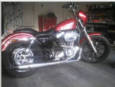
Sprocket cover mod by Big Al Repro K-type cover welded into a 1989 sprocket cover. Stock brake pedal with a fabricated steel backing plate and rod plunger to run a Brembo PS11 master cylinder. 4)
