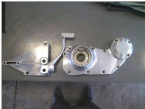
Sprocket cover mod by Big Al Repro K-type cover welded into a 1989 sprocket cover. Stock brake pedal with a fabricated steel backing plate and rod plunger to run a Brembo PS11 master cylinder. 4)
