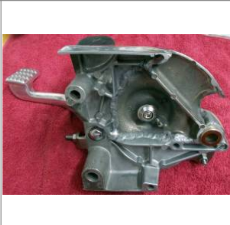
Sprocket cover mod by Big Al Repro K-type cover welded into a 1989 sprocket cover. Stock brake pedal with a fabricated steel backing plate and rod plunger to run a Brembo PS11 master cylinder. 4)
