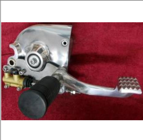
Sprocket cover mod by Big Al Repro K-type cover welded into a 1989 sprocket cover. Stock brake pedal with a fabricated steel backing plate and rod plunger to run a Brembo PS11 master cylinder. 4)
