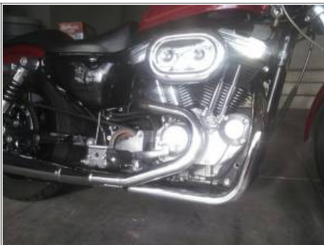
Sprocket cover mod by Big Al Repro K-type cover welded into a 1989 sprocket cover. Stock brake pedal with a fabricated steel backing plate and rod plunger to run a Brembo PS11 master cylinder. 4)
