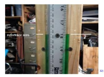
Before the new umbrellas, 3-3/4" (7-1/2" WC) of vacuum was lost while removing the oil cap and the engine died when removing the cap.
