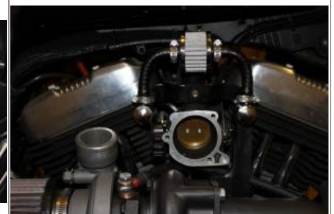
Filter mounted high will receive built up sludge. 14)
