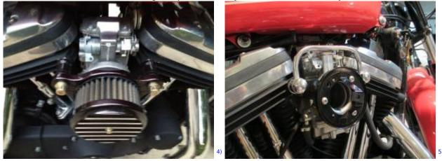
The bracket for the catch can was fabricated from some scrap steel then powder coated.
