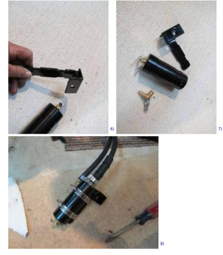
The catch can was mounted to an existing hole in the frame (out of the way between the front lower frame rails).
