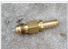
Timing Hole Hose Barb Rig 3/8" NPTx1/4" brass bushing and 1/4"NPTx3/16" hose barb fitting (not necessary but the 3/8" fitting threads were chased with a 5/8"x18 die to remove the thread taper) with a washer and antisieze. Assembly used in timing hole.
