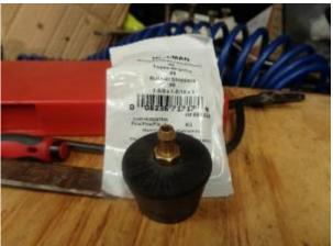
The body was shaved by chucking the fitting into a drill and the plug was spun lightly on top of a rasp clamped in a vise.
