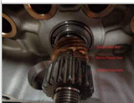
Pinion gear slot aligned with pump gear face. 22)
