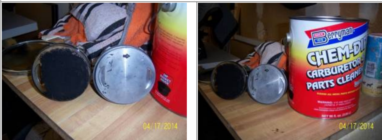
This oil pump soaked overnight to loosen the body to cover gasket. 2)
