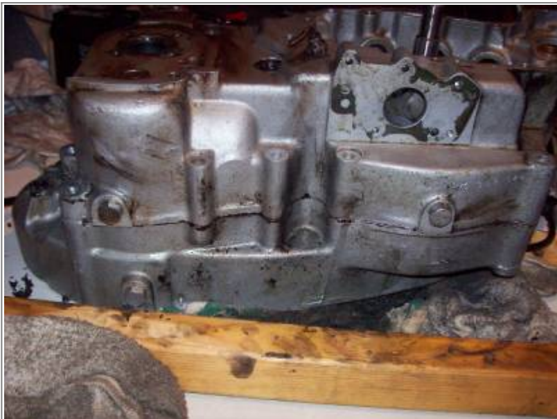
Drain plugs in a '75 case 32)
