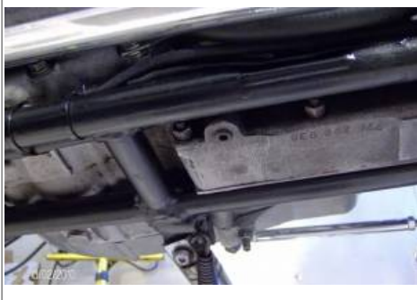
Case & Tranny Drain Plugs on a 1978 engine 53)
