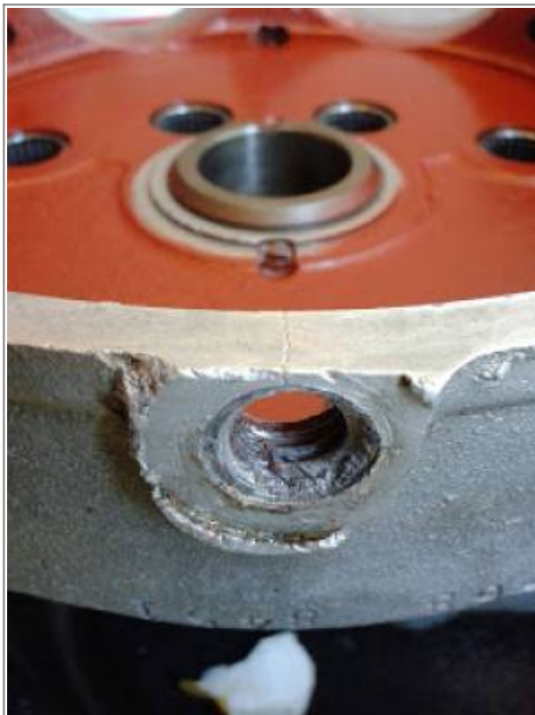
Cracked case at the crankcase drain plug on a 1968 XLCH 49)
