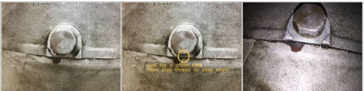
Leak around oil drain plug. 46) In this instance, the case seam appears to be weeping oil.
