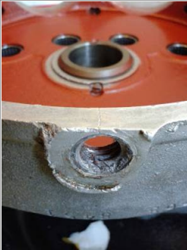
Cracked case at the crankcase drain plug on a 1968 XLCH 48)
