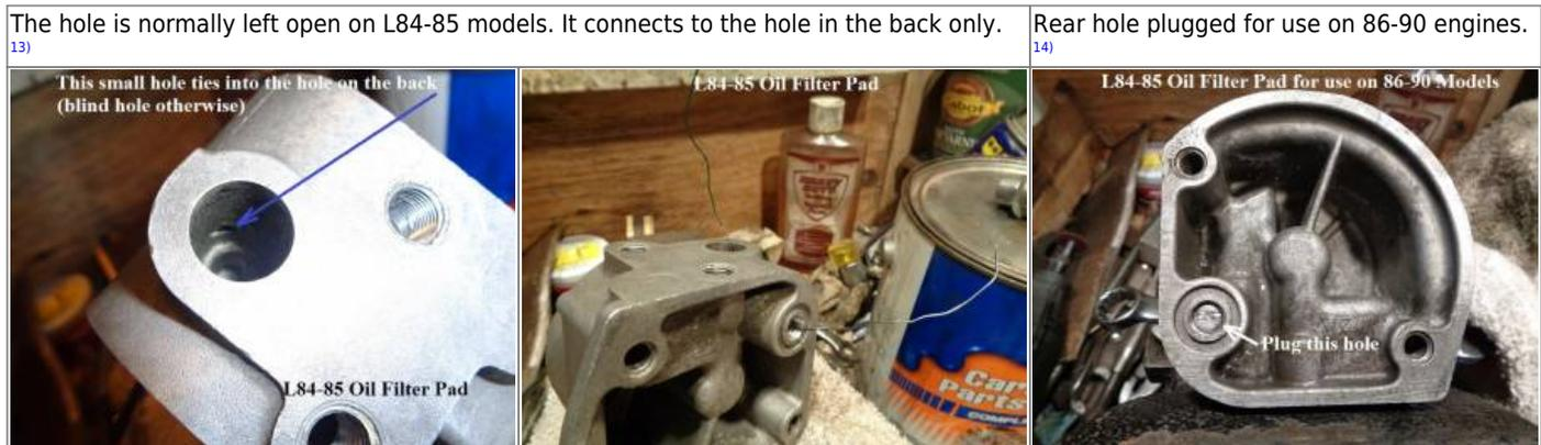
Line routing is the same as in the 86-90 filter pad with exception that the outlet hole for filtered oil has 1/8" NPT threads.
