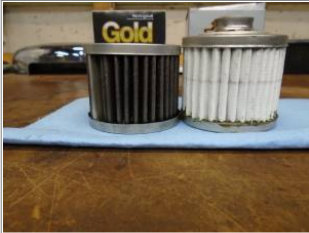
The HD filter has more filter media. Napa 7148 (L) - HD 63731-99A (R) 11)
