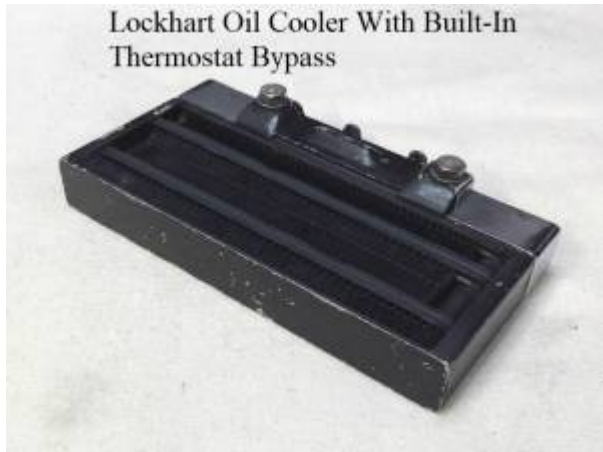
Lockhart Oil Cooler With Built-In Thermostat Bypass
