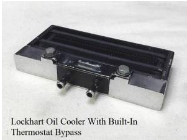
Lockhart Oil Cooler With Built-In Thermostat Bypass
