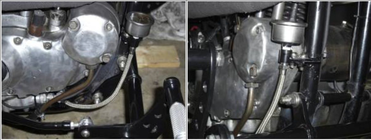
Oil pressure gauge on a 74 model mounted down low by the forward controls 25)
