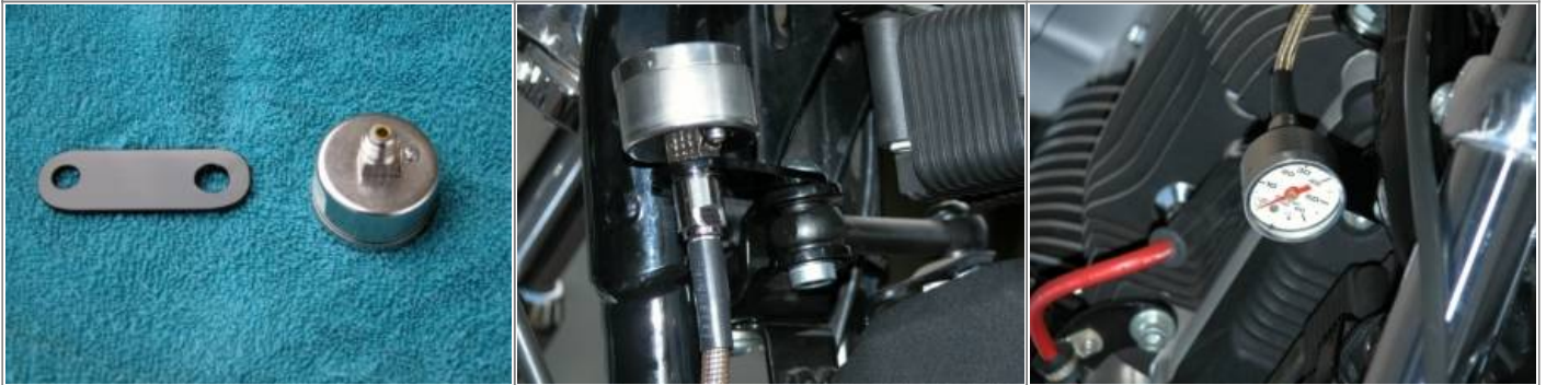
Gauge mounted on the enricher bracket with an L shaped bracket from an old carb support. 37)
