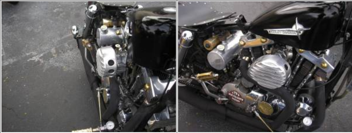
Oil pressure gauge on a 74 model mounted down low by the forward controls 25)
