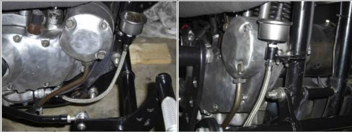
Oil pressure gauge on a 74 model mounted down low by the forward controls 25)
