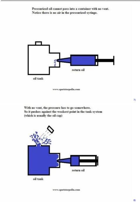
Since it's not the oil pump scavenger's job to separate the oil/air mist, both crankcase pressure and oil end up in the oil tank. 9)
