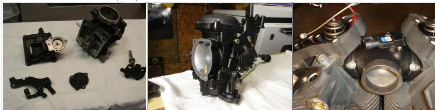
Individual parts powder coated and installed with the intake manifold done as well. 11)
