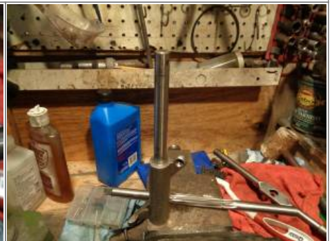
You can see beginning reamer cut in the first pic below. As the reamer came thru, it didn't cut in the middle as well as it did in the beginning. This left an app .0003" hump in the middle of the bushing. Some of that came out with a short lapping with 220 grit.
