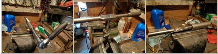
The reamer was sent back through with resistance noticed. But no more shavings ended up on the reamer. So the reamer is done cutting even though the shaft will not slide into the bushing and probably from one or more conditions above. The reamer theoretically cuts a center hole thru / from both bushings. However, the hole now has to be lapped to widen the 'centered' hole to accept the shaft. (in proper clearance) <sup>26)</sup>
