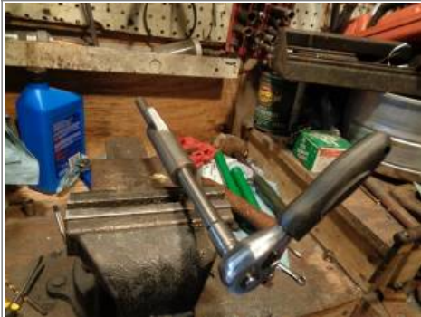
The reamer was sent back through with resistance noticed. But no more shavings ended up on the reamer. So the reamer is done cutting even though the shaft will not slide into the bushing and probably from one or more conditions above. The reamer theoretically cuts a center hole thru / from both bushings. However, the hole now has to be lapped to widen the 'centered' hole to accept the shaft. (in proper clearance) 26)
