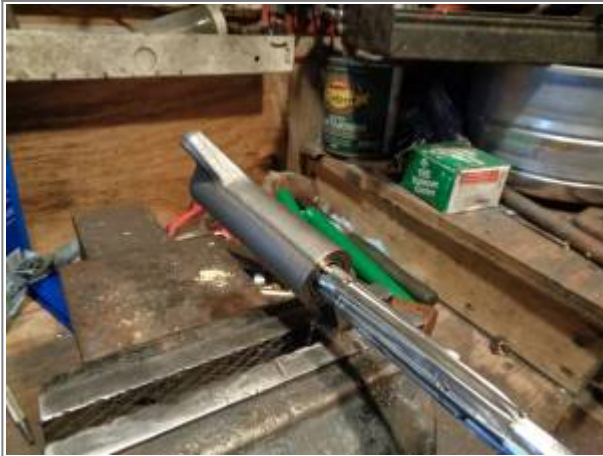
A 12 mm socket and wrench can be used to turn the reamer. But a standard tap wrench works good. You can see how much was cut out during reaming. 25)
