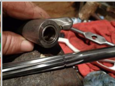
You can see beginning reamer cut in the first pic below. As the reamer came thru, it didn't cut in the middle as well as it did in the beginning. This left an app .0003" hump in the middle of the bushing. Some of that came out with a short lapping with 220 grit.
