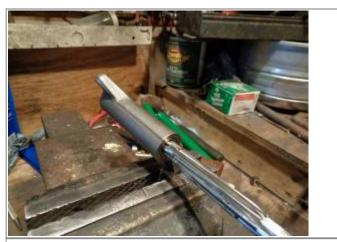
A 12 mm socket and wrench can be used to turn the reamer. But a standard tap wrench works good. You can see how much was cut out during reaming. <sup>25)</sup>
