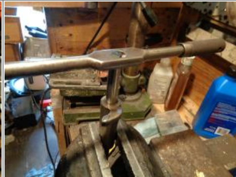
The reamer was sent back through with resistance noticed. But no more shavings ended up on the reamer. So the reamer is done cutting even though the shaft will not slide into the bushing and probably from one or more conditions above. The reamer theoretically cuts a center hole thru / from both bushings. However, the hole now has to be lapped to widen the 'centered' hole to accept the shaft. (in proper clearance) 26)
