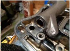
If so, the bushing isn't home yet. The nut below was installed alone to pull the bushing in the rest of the way.
