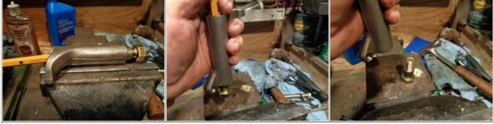
The newly cut threads will be damaged once the bushing is removed. This makes the initial threading important for best results. 14)
