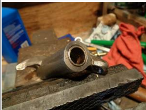
You can see beginning reamer cut in the first pic below. As the reamer came thru, it didn't cut in the middle as well as it did in the beginning. This left an app .0003" hump in the middle of the bushing. Some of that came out with a short lapping with 220 grit.
