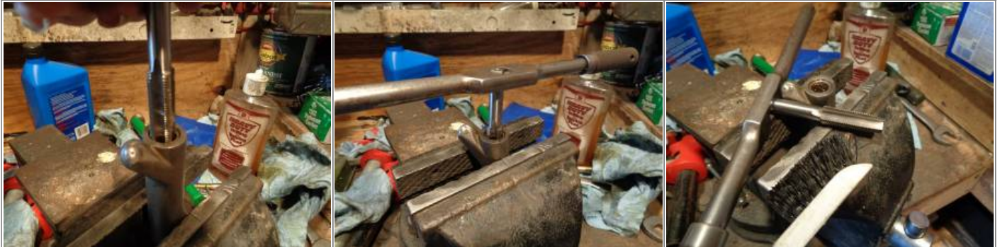
Clean the threads in the bushing for the 9/16" bolt. The vise won't hurt the rocker arm. 11)
