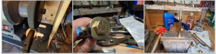
One modified washer, then the rocker installed over the bolt. Adjust the washer to fit around the arm. Then add the bushing, second washer and nut. Make sure the split in the washer is facing up as in the installed position. At this point, it doesn't matter about the position of the notch made in the second washer.
