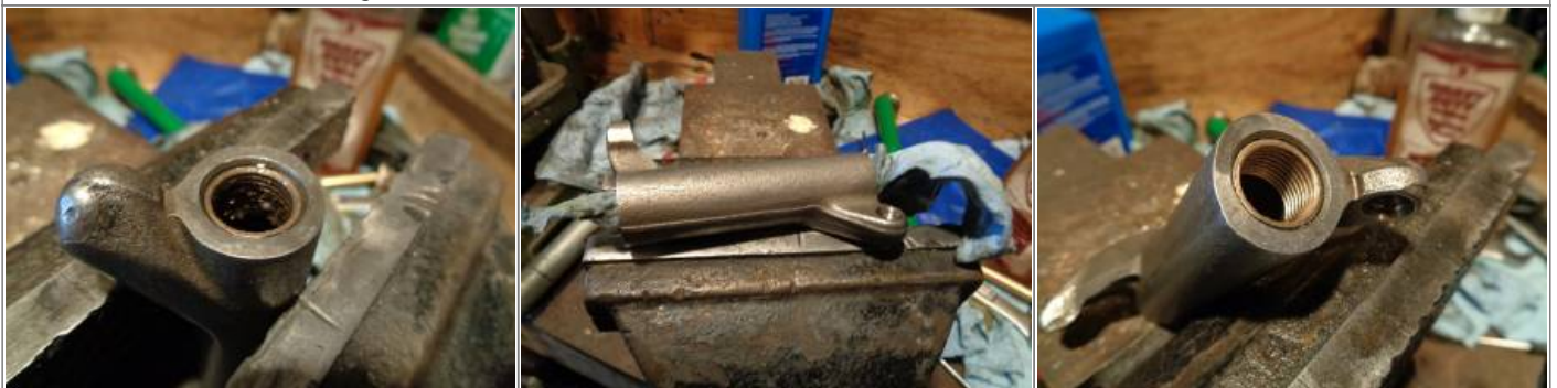
Run the 9/16" bolt in for the length of the bushing. It takes a couple good hits to initially move the bushing. 12)
