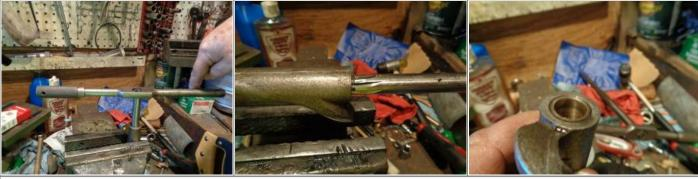
The shaft did slide in with light resistance but repeated turns with the reamer also created heat in this spot. It still needed to be lapped for greater clearance.
