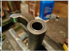
If needed, the end of the bushing can be filed down flush to the rocker arm. Place a straightedge across the assembly to ensure it's flat
