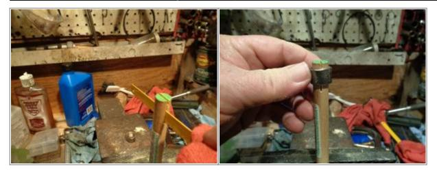
Initially cut a piece of sandpaper to go one full revolution around the dowel. 28)
