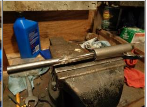
The reamer was sent back through with resistance noticed. But no more shavings ended up on the reamer. So the reamer is done cutting even though the shaft will not slide into the bushing and probably from one or more conditions above. The reamer theoretically cuts a center hole thru / from both bushings. However, the hole now has to be lapped to widen the 'centered' hole to accept the shaft. (in proper clearance) 26)
