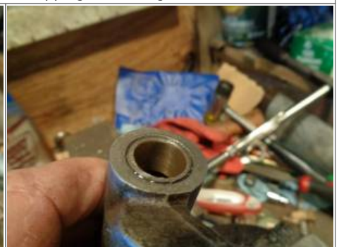
This revealed a dark ring where the reamer was binding but not cutting.
