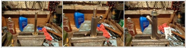
Turn the bolt in with the wrench in one hand and the other hand on the rocker (as you would with a torque wrench).
