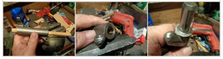
Repeat until the clearance is correct at each bushing / shaft end (individually measured and matched per side).
