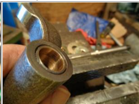
This revealed a dark ring where the reamer was binding but not cutting.
