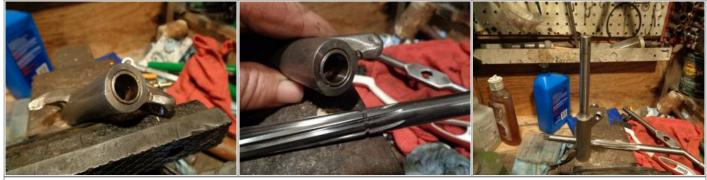
You can see beginning reamer cut in the first pic below. As the reamer came thru, it didn't cut in the middle as well as it did in the beginning.
