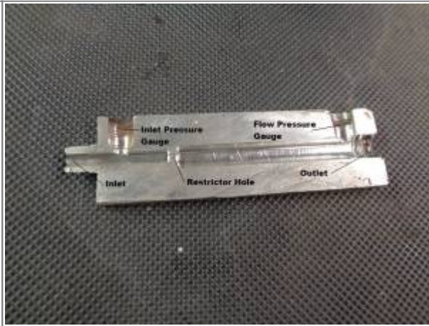
Cut-away showing the air path 16)
