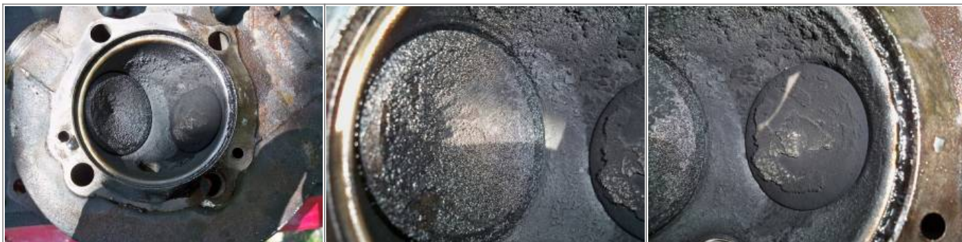
Excess carbon between valve and seat causing a leak on this 73 XLCH. 37)
