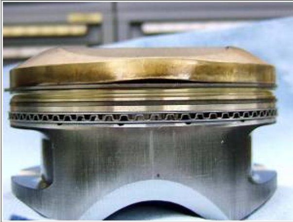
This piston is just about to break from too much cylinder pressure. This is from a race motor using Nitromethane 42)
