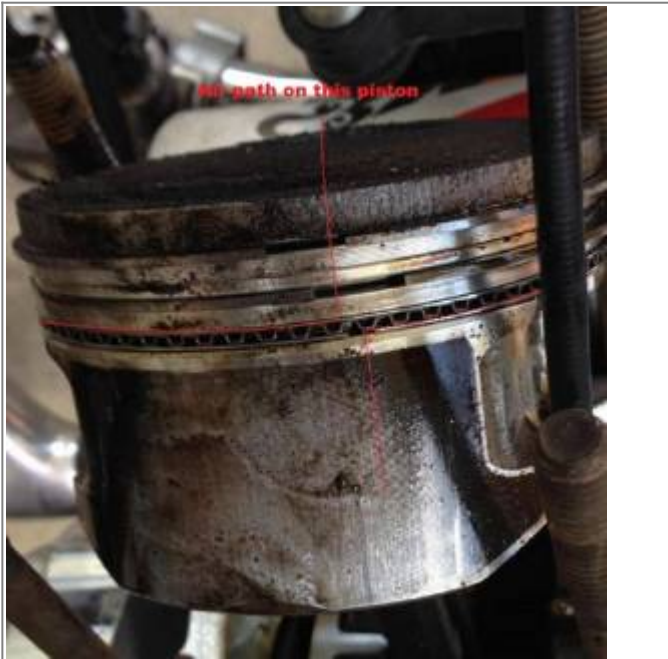
Top 2 rings are lined up vertically on this piston 41)
