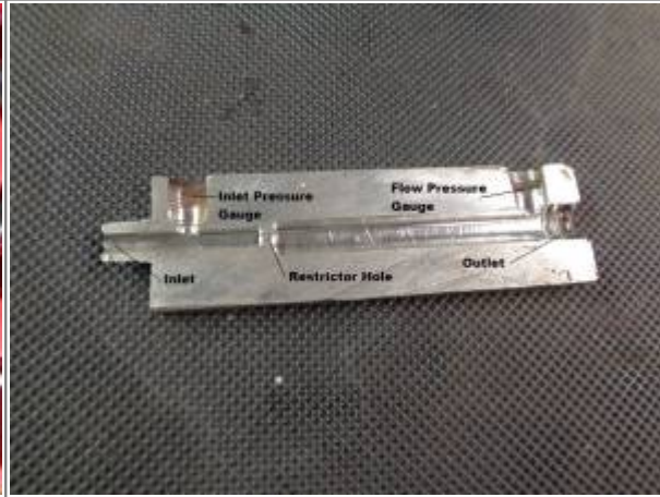
Cut-away showing the air path 16)
