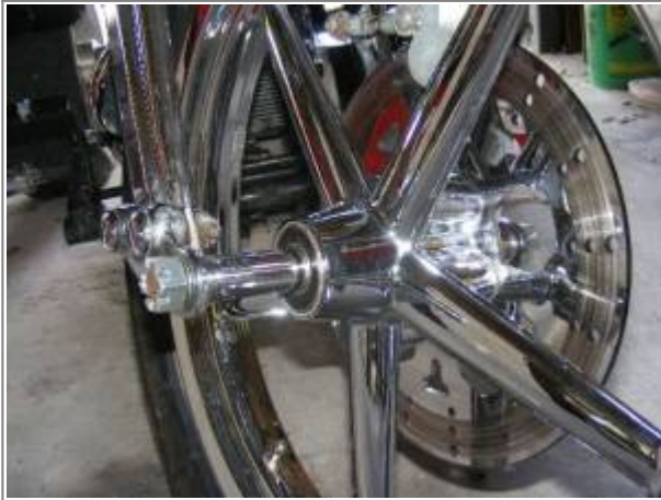
Polished stainless steel axle spacers 37)
