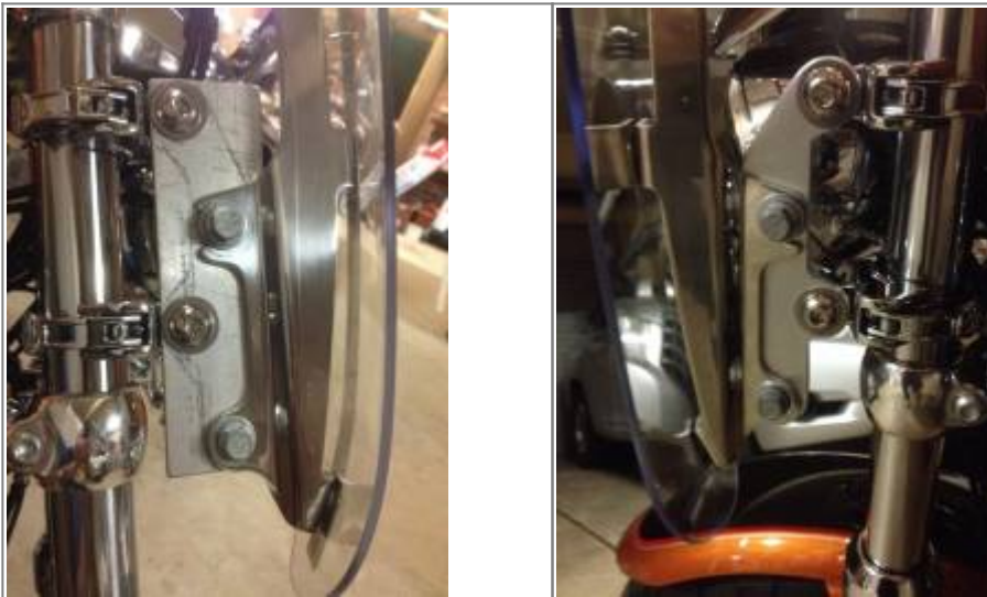
Homemade windshield lowering brackets with a polished brushed finish. 38)
