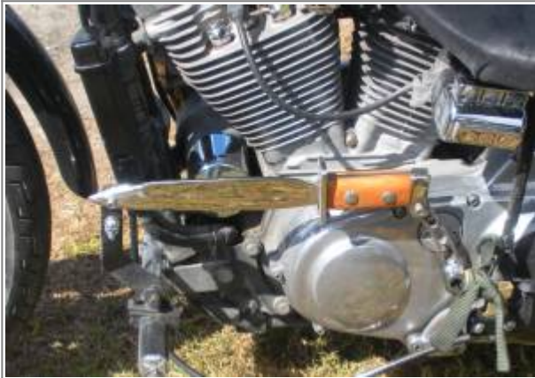
Shifter linkage shaped like a knife 35)
