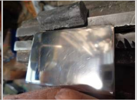
The black stick when rubbed across the metal will scratch it.
