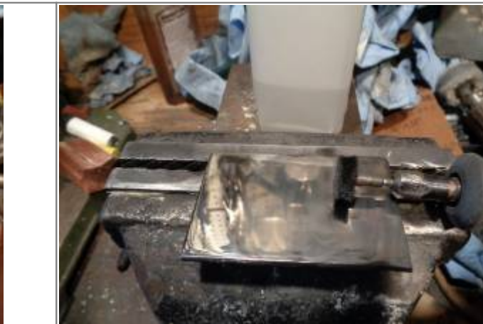
However, the excess polish buildup was caused by loading too much polish on the wheel. A wheel rake was used to remove the excess polish which made it more manageable on the next run.
