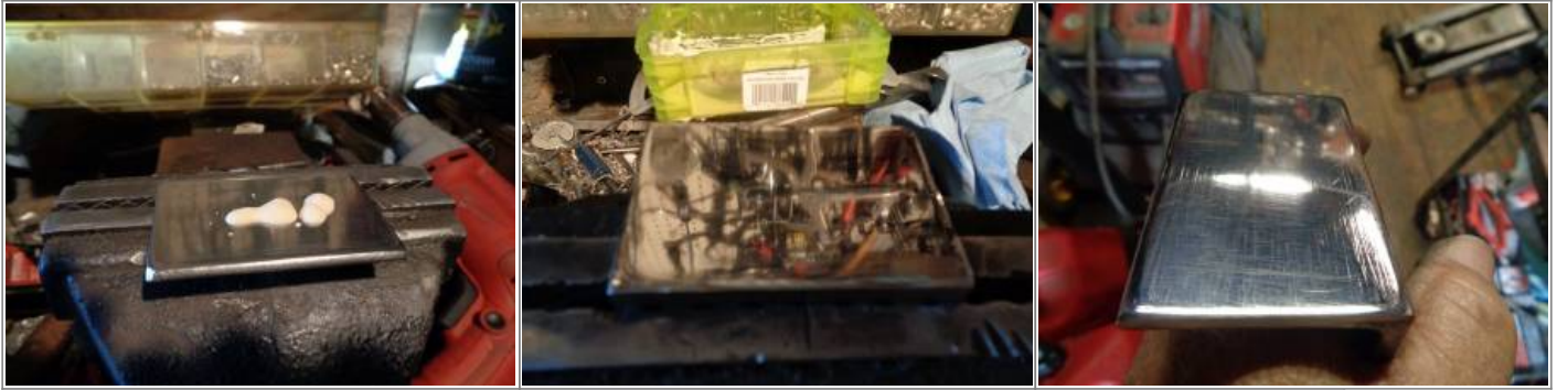
3m applied with a Dremil tool and a felt disc leaves a better shine.
