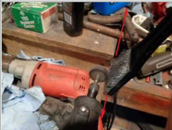
However, the excess polish buildup was caused by loading too much polish on the wheel. A wheel rake was used to remove the excess polish which made it more manageable on the next run.
