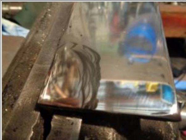
However, the excess polish buildup was caused by loading too much polish on the wheel. A wheel rake was used to remove the excess polish which made it more manageable on the next run.
