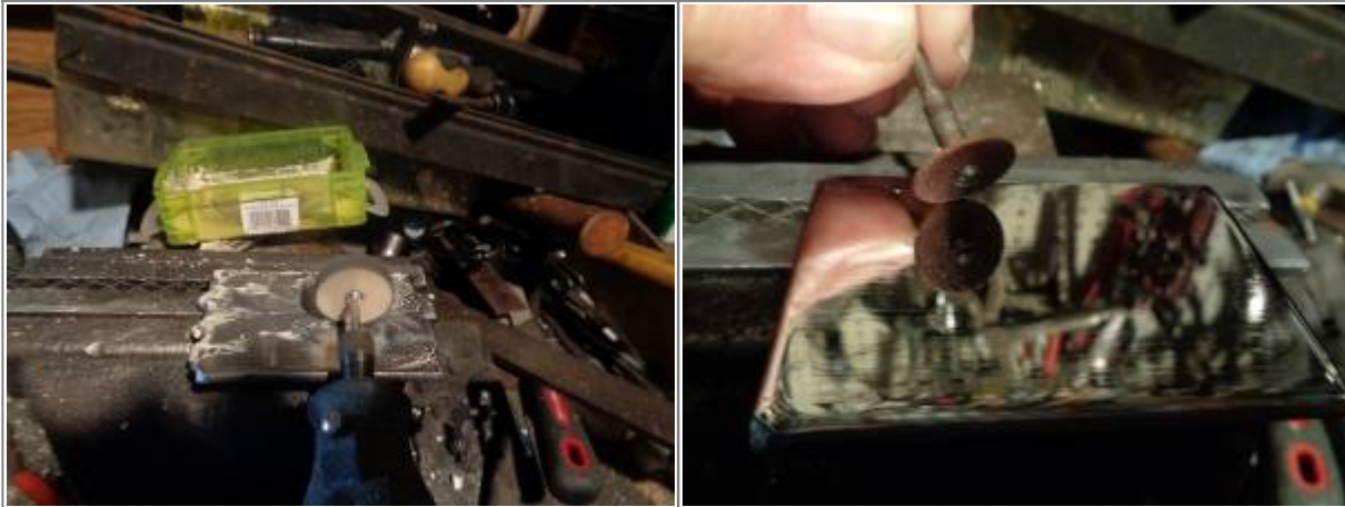
Then, white polishing compound was used from a Harbor Freight kit. Held in a vise for easy access. But the scratches are still too deep.
