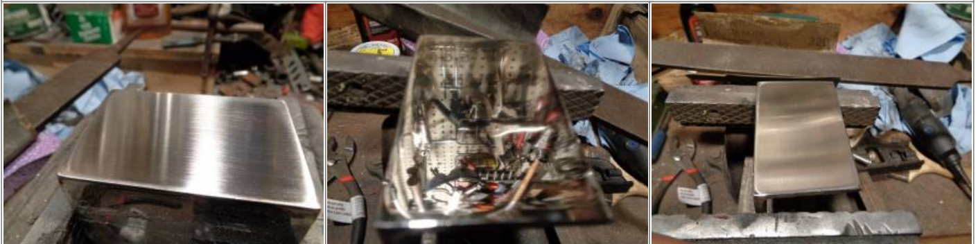
After using 400 grit, the lines are fading out but too much pressure was applied while sanding and light scratches appeared. They still won't polish out with white compound.
