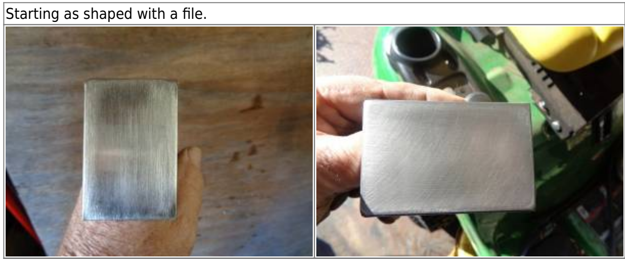
A course sanding block smoothed it out some but it's too flexible and began rounding the corners.
