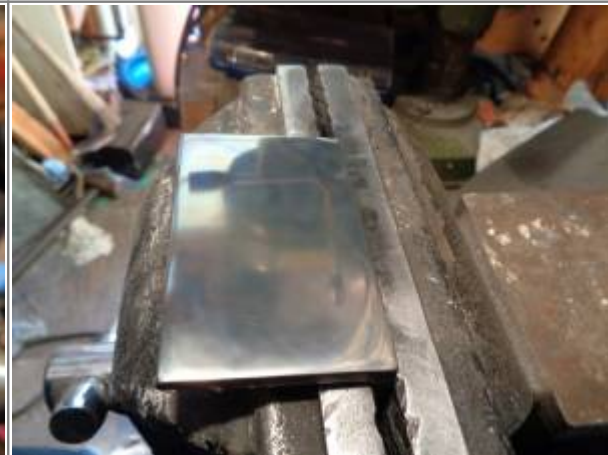
However, the excess polish buildup was caused by loading too much polish on the wheel. A wheel rake was used to remove the excess polish which made it more manageable on the next run.
