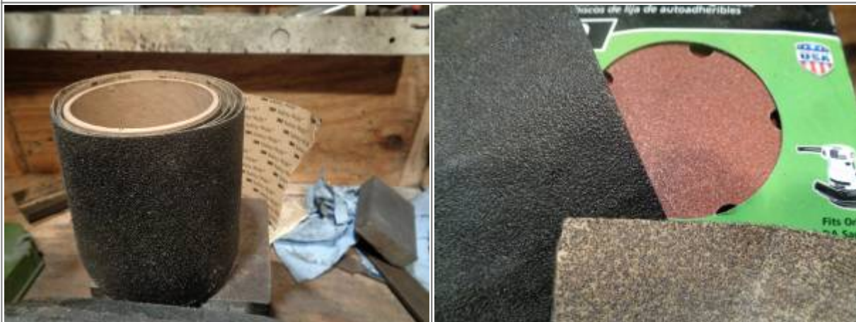
This is sold as "3M Safety Walk" (applied on steps to keep your feet from slipping). It makes for a good rough sandpaper and looks to rival the 60 grit paper in front.
