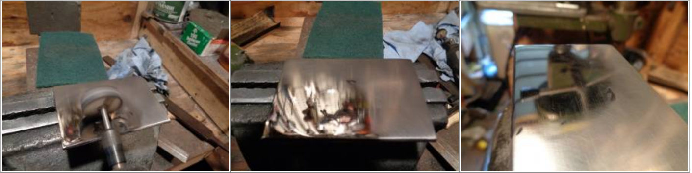
The aluminum oxide disc was a bad idea. It knocked down some of the valleys but dimpled the surface
