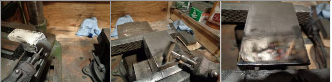
This is sold as "3M Safety Walk" (applied on steps to keep your feet from slipping). It makes for a good rough sandpaper and looks to rival the 60 grit paper in front.
