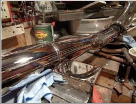
Sanded back down by hand only with wet 400, dry 600 and 1200 grit. Then wet sanded with steel wool and polished with the black stick.
