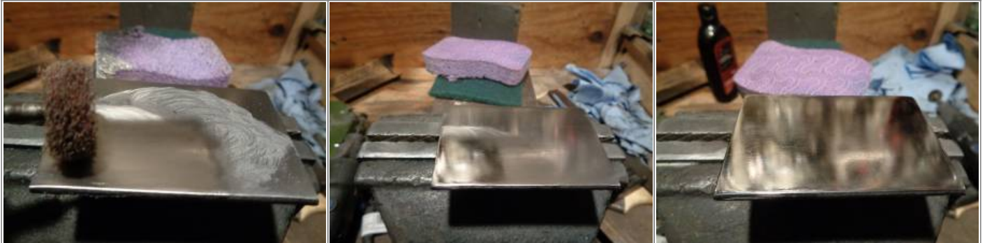
The surface was then wet sanded with 320 grit and polished with white compound. The surface feels like glass but the lines are still in it.
