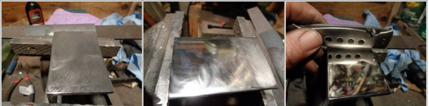
A cloth wheel on a drill was useless and added more scratches.
