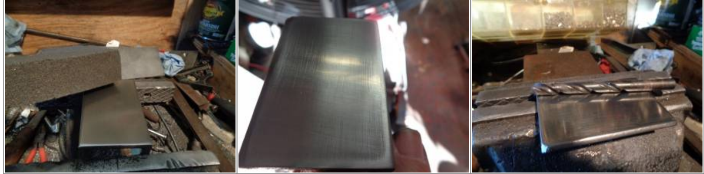
3M polishing compound applied with the sanding block.
