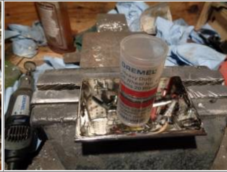
Sanded back down by hand only with wet 400, dry 600 and 1200 grit. Then wet sanded with steel wool and polished with the black stick.
