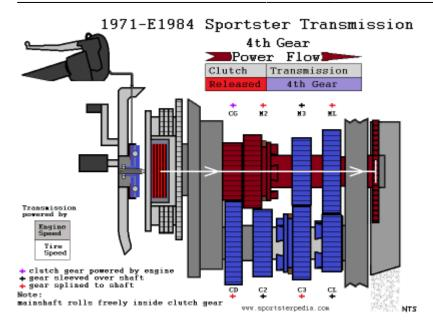
The animated image below shows how the gears are positioned and then moved to attach to their mating gears throughout the gear range.
