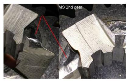
This is the female "slot" side of MS 2nd showing the rounded corners from the Clutch Gear backing out of it.
