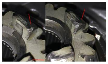
These are different dogs on the same clutch gear. The damage is obvious on the dogs. Also note the damage is different on each dog
