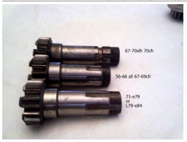
In this pic, I added a gear with the extension to the lineup.
