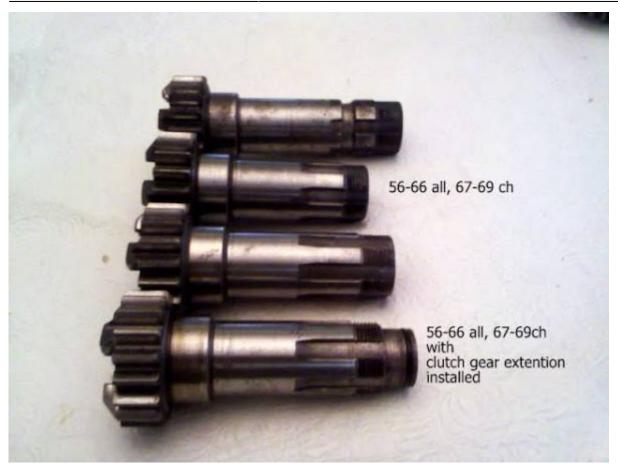
The extension is part of the dry clutch sealing system.
