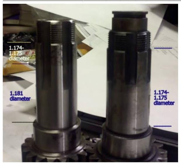
The AP gear is very hard. 60rockwell c scale.
