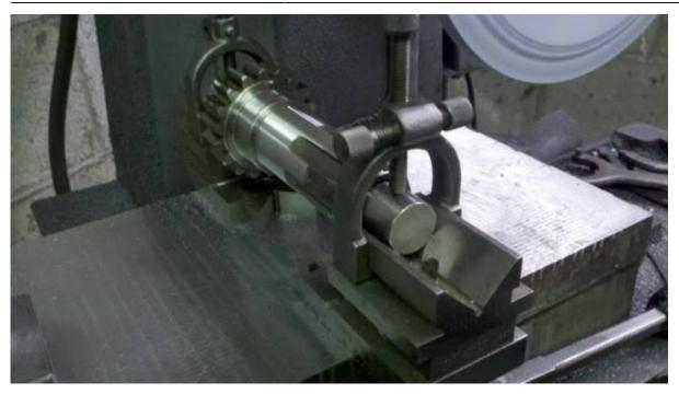
While grinding, the wheel will want to spin the gear. I use my hi-tech workpiece speed governor to keep things under control.
