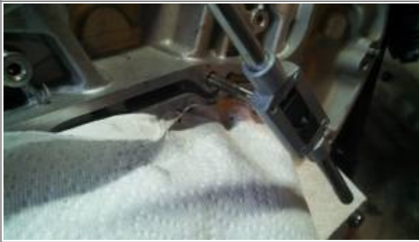
Chasing cam cover threads. 12)
