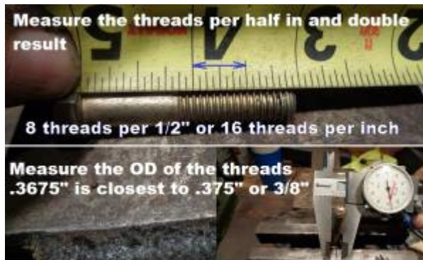
Field measuring 3/8\" x 16 Bolt threads
