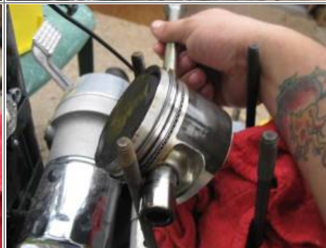
A 1/2x13 carriage bolt set into the pin hole and either pushed or light threading motion with pressure applied to remove the wrist pin. 8)
