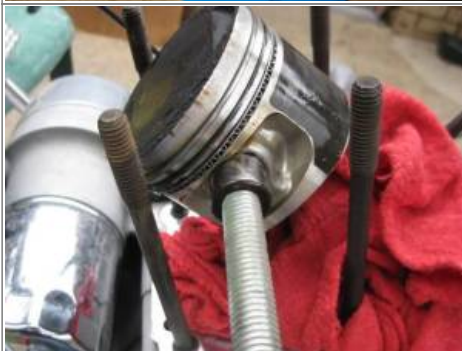
A 1/2x13 carriage bolt set into the pin hole and either pushed or light threading motion with pressure applied to remove the wrist pin. 8)
