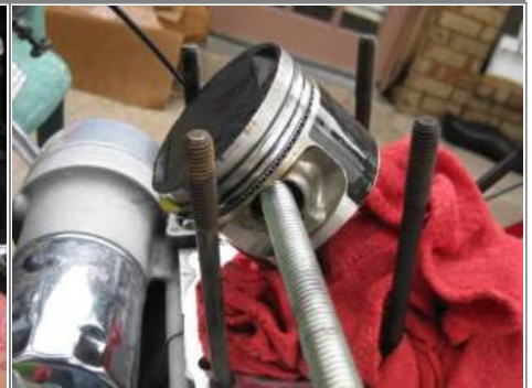
Wrist pin bushing installer: 3/4" bolt with two washers and a nut. 7)
