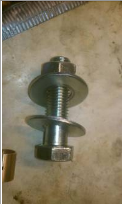
Wrist pin bushing installer: 3/4" bolt with two washers and a nut. 7)
