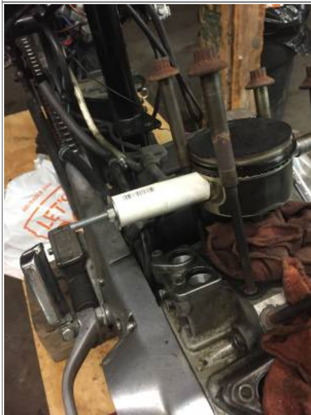
Home made wrist pin removal / installation tool. 5/16" all thread, 2 fender washers, two nuts, two PVC spacers and two 1/2" sockets. 4)
