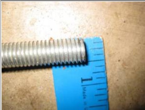
Wrist pin bushing installer: 3/4" bolt with two washers and a nut. 7)
