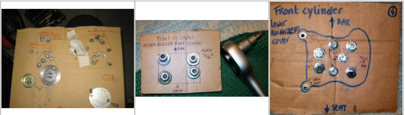
Protecting rocker box screws and parts 11) 12) 13)
