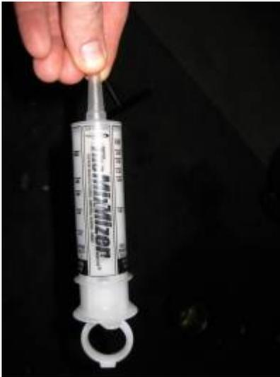
This is an oil / fuel mixing syringe for 2 cycle engines that can be purchased for under \$5 at most automotive departments and parts stores. <sup>1)</sup>
