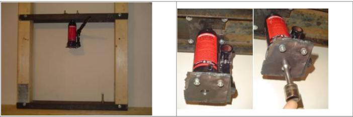
Can be made from whatever you find at the scrap yard, this was made from steel channel bolted to the 2x4s.
