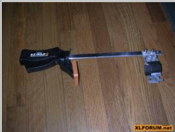
Homemade fork spring compressor 2)
