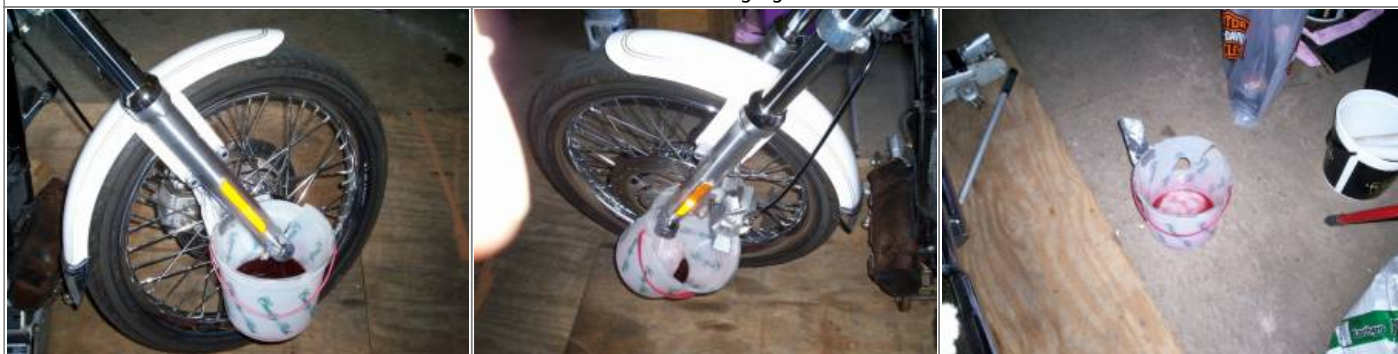
Drain bucket for changing fork oil. 15)
