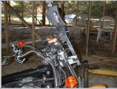
Attach the conduit clamp to the fork. 3)
