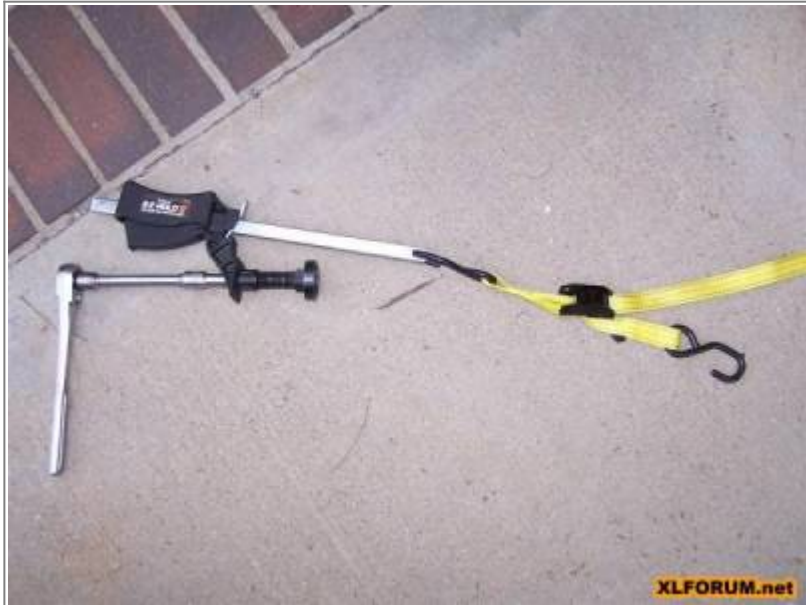
Homemade fork spring compressor 8)
