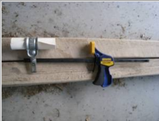
Homemade fork spring compressor 5)
